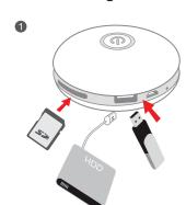
You can insert SD Card into the SD Card Slot, or plug-in your USB or Portable Hard Drive through the USB Port.
